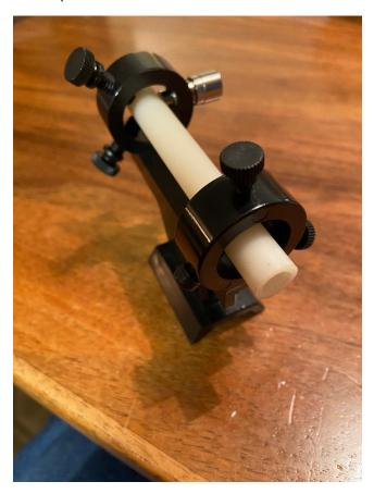
The plastic pipe is 4 inches long and has a hole through it ¼ inch in diameter. This hasn't been tested out yet but we believe it has a field of view slightly larger than the full moon. There is no cross hair so there may be some concern with parallax. The mount would cost less than \$20.
